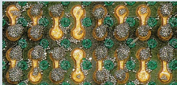
0.3 mm CSP printing: Competitive paste's poor transfer efficiency results in high solder volume variability and the potential for defects.
