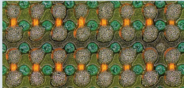
0.3 mm CSP printing: GC 10's high transfer efficiency results in low solder volume variability.
